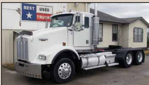
1999 KENWORTH T800 N14 Cummins 460 HP, 10 Spd, 3.90 Ratio, 204" WB, Eng. Brake, 8 Bag Air Ride Susp., 22.5LP Tires, Alum./Steel Wheels, Tandem Axle, $26,500 , Stk# 2057
